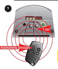
Press and hold the remote control button the press the adjustement pushbutton briefly to memorise the remote control buttons.
